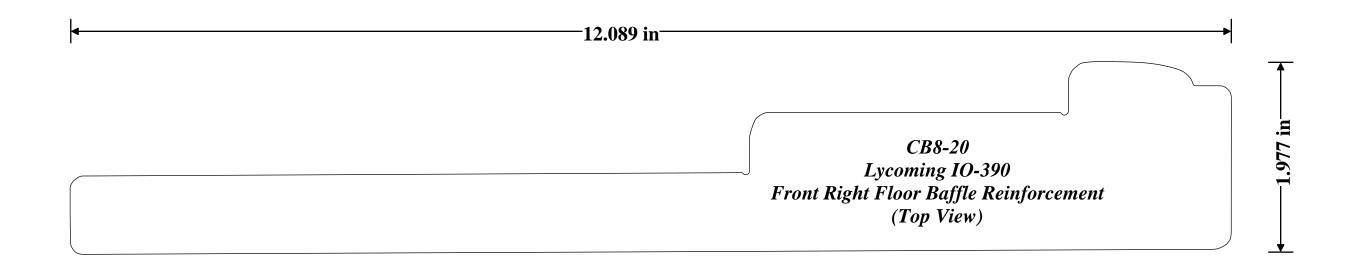
"CB8-20" Lycoming IO-390 Front Right Floor Baffle Reinforcement
